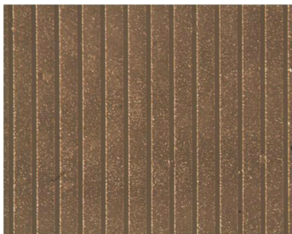
Figure 8. Photograph of a 100\text{-}\mu\text{m} -wide \text{Er}^{3+} -doped cPVP film by lift-off process.
